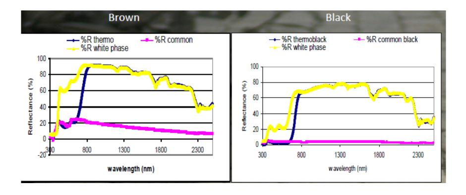
Thermochromic coatings present a high reflectivity both in the visible and infrared spectrum, while they present very strong absorption in the nearultraviolet range of the spectrum.
