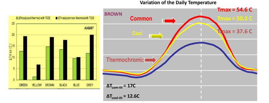
■ Thermochromic coatings exhibit higher solar reflectance values and lower temperatures compared to common and cool coatings of the same colour
