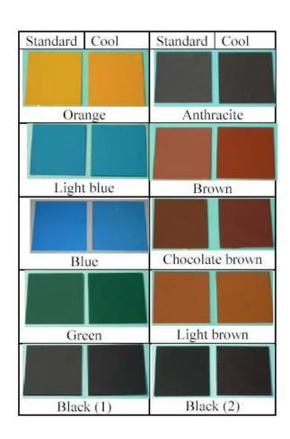
■ The optical properties and the thermal performance of 10 prototype cool colored coatings, prepared at the University of Athens using near-infrared reflective color pigments are tested in comparison to color- matched, conventionally pigmented coatings in an effort to investigate the ability of the cool colored coatings to maintain lower surface temperatures than conventionally pigmented color-matched coatings under sunlight and during the night during both summer and winter
