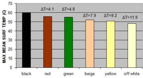
■ Cool Asphaltic materials present a much higher reflectivity and also a lower surface temperature compared to conventional asphalt materials.
